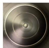
Top of Jetted Check Valve
